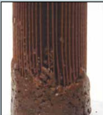
**Sediment** - *Granules, sediment in the folds of the filter.*
