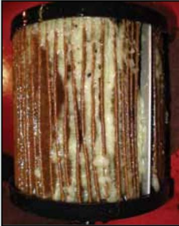
**Paraffin Wax** - *Clean filter and hazy fuel. Wax substance in the folds of the filter in temperatures at or below the cloud point.*
