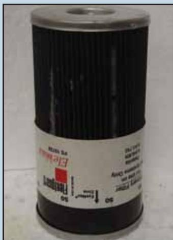
**Microbial Contamination -** *Slimy filter with odor, or a black, slimy filter with or without odor.*
